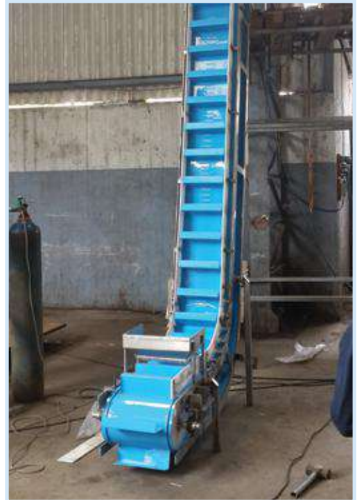
Fixed conveyor side wall
